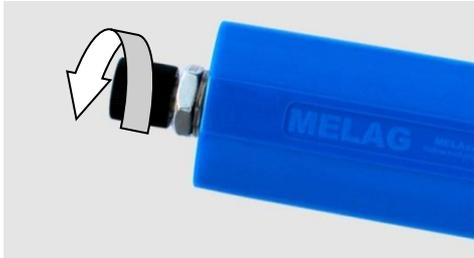
1. Unscrew the cap from the helix test body.
